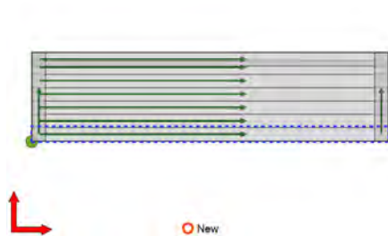
Figure 66: Example of parallel scan pattern
