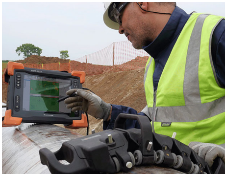
Figure 1: Operator performing in-field data analysis during a pipeline inspection using a Spyn™ ECA probe, Reddy® instrument, and Magnifi GO software.
