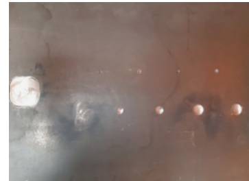
ECA custom probe on various round bottom holes over a 30 mm rubber tile
