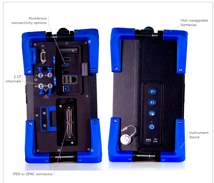
Figure 2: Annotated breakdown of TOPAZ64 showing its key features.
