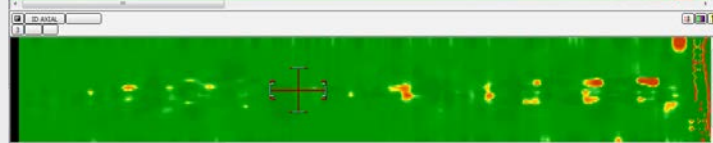
Axial ID defects
