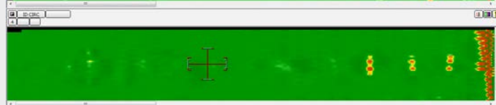
Circumferential ID defects
