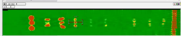
Circumferential OD defects
