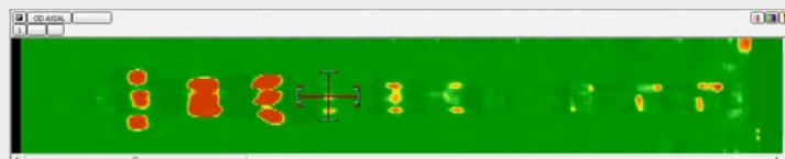
Axial OD defects
