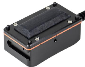
The result is a probe composed of six rows of coils, for a total of 126 multiplexed coils on a flexible PCB, yielding close to 128 ECA channels. This configuration gives the probe enough resolution to reliably detect the target incomplete penetration and other small defects.
