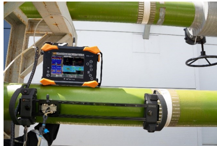
Left to right: R-Scan Array on dome end and LYNCS CM for straight pipework
