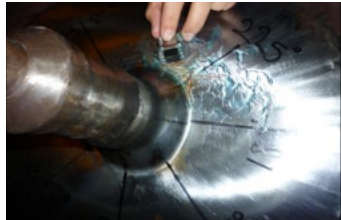
Figure 12: Probe orientation for defect located in position 225°
