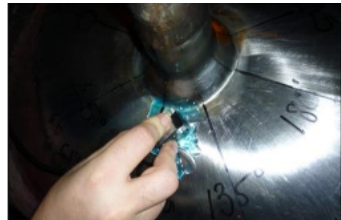
Figure 14: Probe orientation for defect located in position 135°
