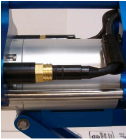
FIGURE 11: LUBRICATE AND PUSH ON CONNECTOR
