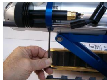
FIGURE 10: POSITION LIGHT AND TIGHTEN
