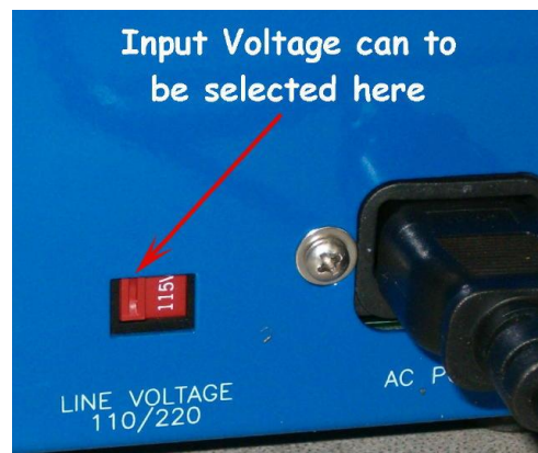
FIGURE 1: AC LINE VOLTAGE SELECTION
