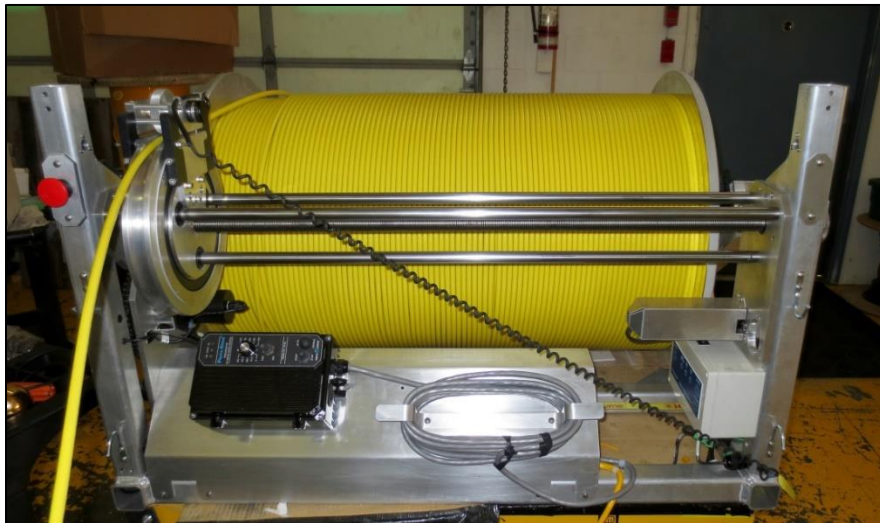
FIGURE 16: CABLE WRAPS SHOULD BE EVEN AND TIGHTLY SPACED
