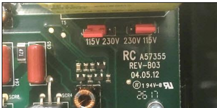
FIGURE 6: 115/230V INPUT SELECTION JUMPERS (115V POSITION)
