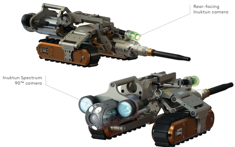
Sensor Integration: Nondestructive testing tools integrate with the Versatrax 150™ Analog for remote sensing and tooling activities
