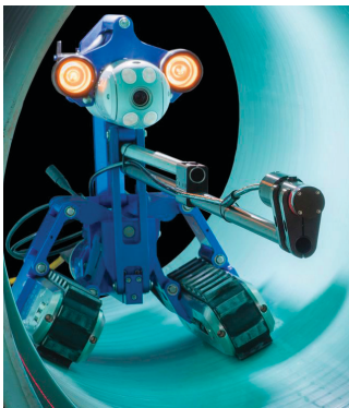
Sensor Integration: Nondestructive testing tools integrate with the Versatrax 150™ Analog for remote sensing and tooling activities
