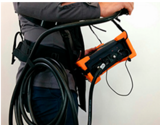
Figure 8-17 Belt-slinging probe cable
