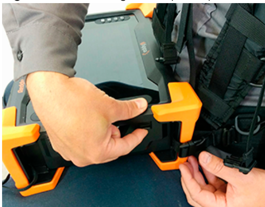
Figure 8-14 Closing battery compartment door.
