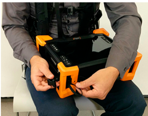
Figure 8-8 Sliding strap loop through bumper hook
