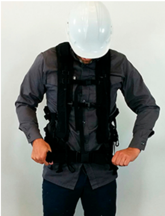
Figure 8-5 Securing the belt
