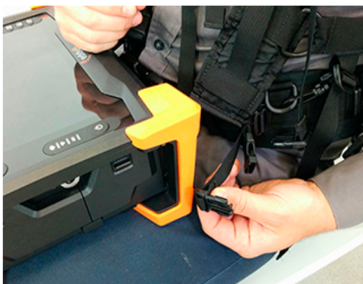
Figure 8-11 Anchor strap on harness belt
