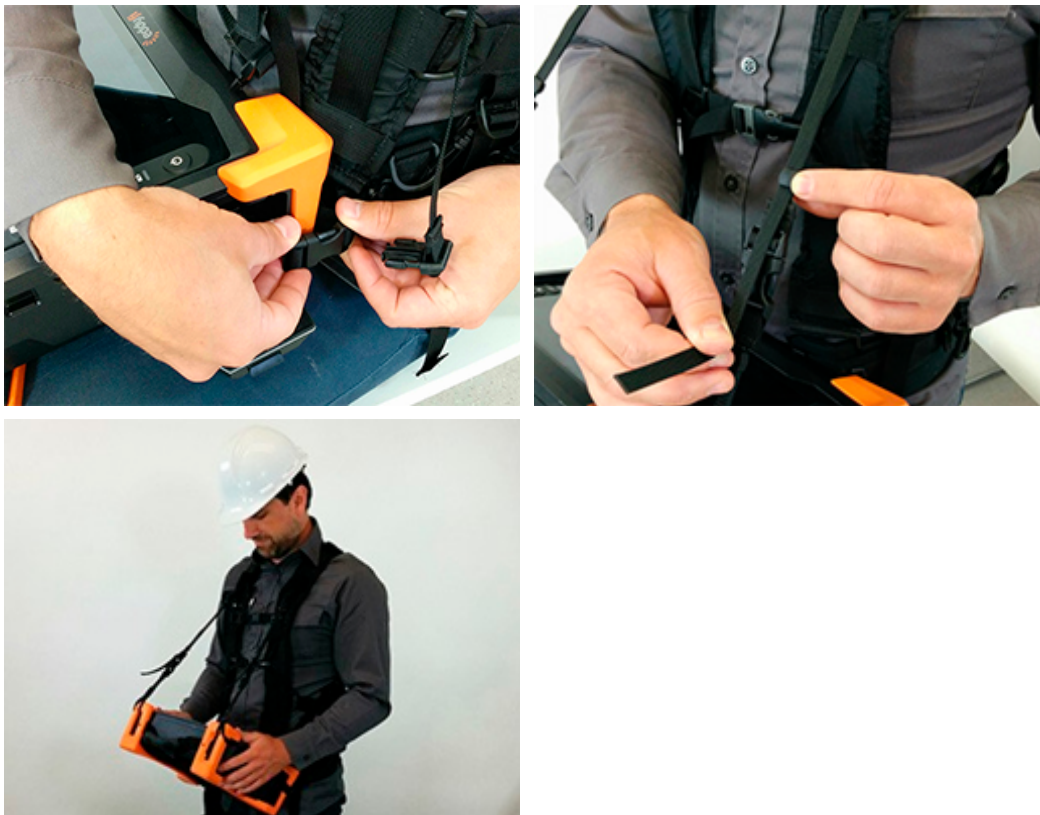
Figure 8-13 Mating battery compartment side anchor strap
