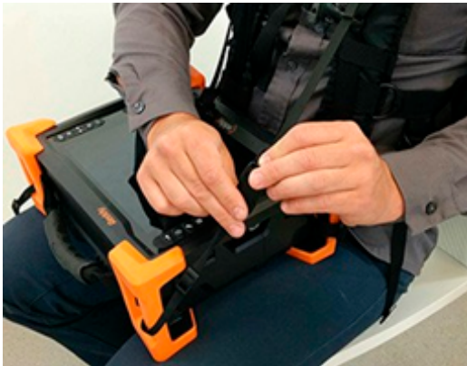
Figure 8-15 Mating shoulder anchor strap
