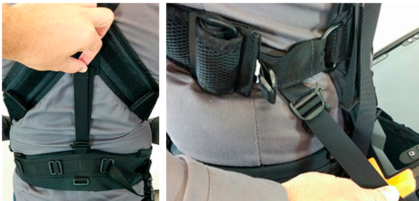
Figure 8-3 Adjusting the belt's height
