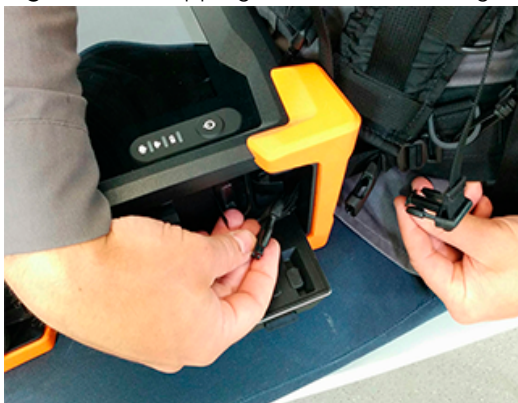
Figure 8-12 Slipping male buckle through bumper
