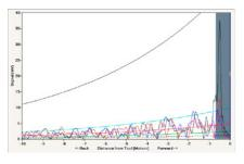
The propagation torsional waves were significantly inhibited by the radial fins along the tube length. This made the detection of the pipe end impossible and the noise of the pipe high.
