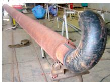
A defect was ground into the center of the pipe and FOCUS+ was used to see
