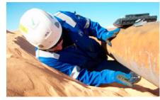
Characterizing external pitting corrosion using pipe pit depth gauges (lever type and dial gauge)
