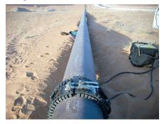
FOCUS<sup>+</sup> guided wave ultrasonic test equipment used to inspect an 45.7 cm (18 in) trunkline of the MLN field in Algeria
