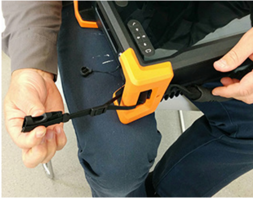
Figure 71 Alternative method of securing anchor strap to bumper
