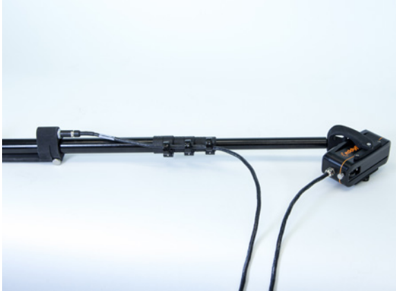
Figure 84 Connecting PEC probe connector to extension pole remote control
