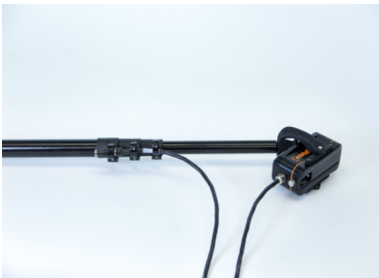
Figure 83 Running PEC probe cable through pole hoops
