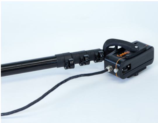
Figure 82 Securing PEC probe to extension pole head
