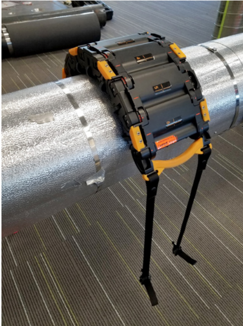
Figure 87 Probe on a pipe with curvature locked
