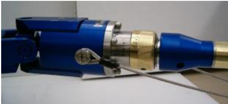
FIGURE 2: TETHER AND TOW CABLE CONNECTION
