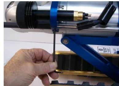
FIGURE 10: POSITION LIGHT AND TIGHTEN
