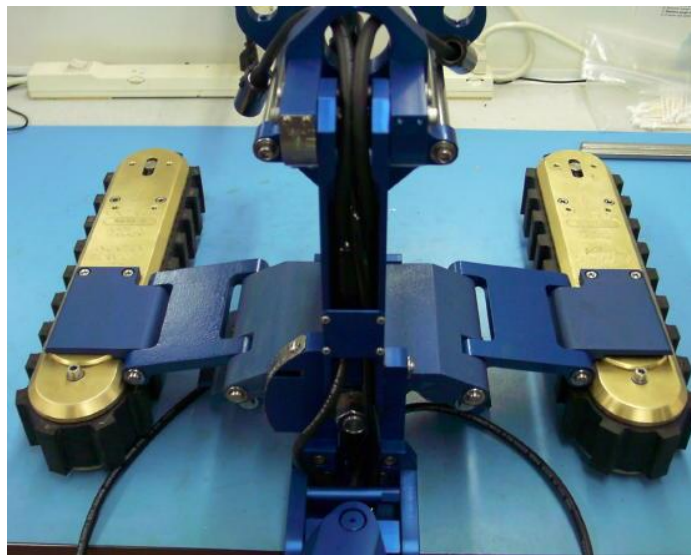
FIGURE 17: TRACKS FLAT ON BENCH – OUTER BRACKETS
