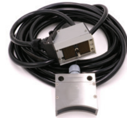
Custom 92-element array for tube and bar testing machines
