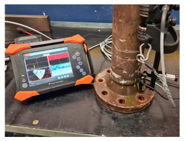
Figure 1: Flange face corrosion assessment with LYNCS  $^{\rm TM}$  and Mantis.
