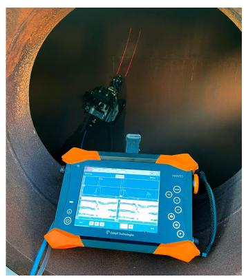
Figure 3: Mantis and VersaTrax™ for remote inspection.
