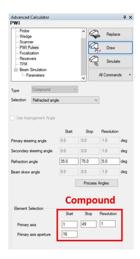
The extent and the number of pulses in the sweep are determined by entering the **Refraction angle Start**, **Stop** and **Resolution** values. If a compound sweep has been defined, the software will automatically optimize the elements to be fired for each angle.
