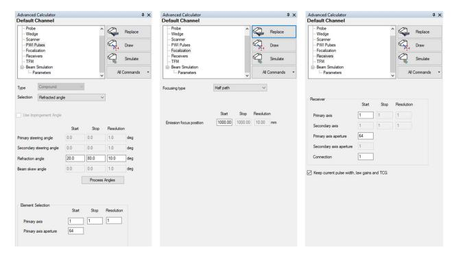
In the **Focalization** tab, the default setting is **Half path 1000 mm**, which basically corresponds to "natural focusing" of the beam or "Plane Wave" excitation.
