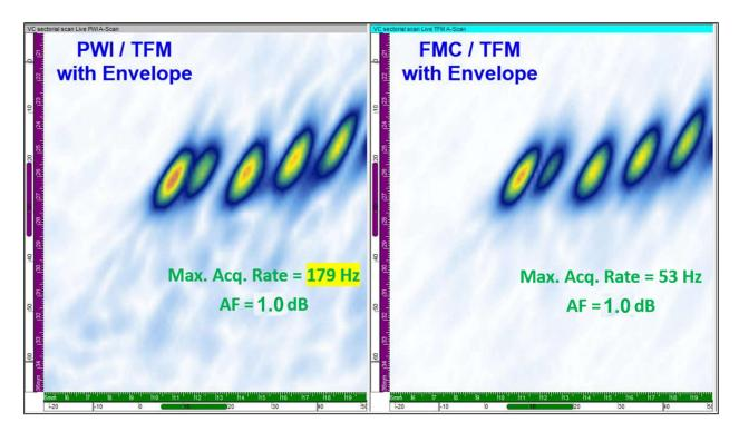
The PWI-TFM images are shown on the left and the regular FMC-TFM images on the right. The Envelope feature is applied in both cases.
