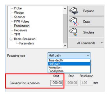
Alternatively, the **Emission focus position** can be set to a smaller value, to insonify the region of interest with focused beams. This corresponds to the physical principle of **Convergent Wave excitation** and **CWI** (**Convergent Wave Imaging**).
