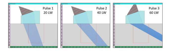
Three pulses are fired sequentially using the full aperture of the probe, and with three different refracted angles. The region of interest (shown in red) is essentially covered by the three naturally focused beams.
