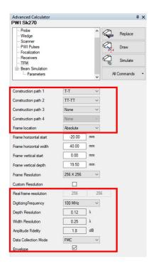
It can also be observed that the UltraVision Classic software now allows to select and process multiple (up to 4) reconstruction paths for a single FMC or PWI firing sequence. In this user case, 2 reconstruction paths have been selected:
