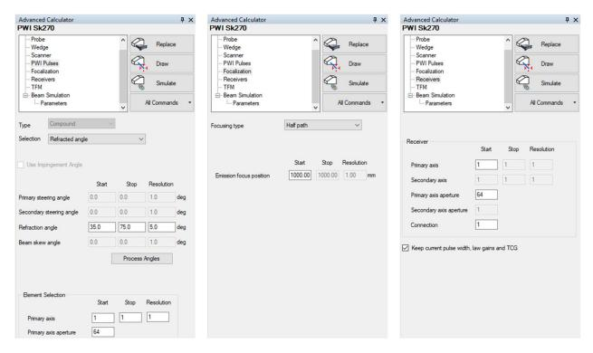
In the **Focalization** tab, the default setting is **Half path 1000 mm,** which basically corresponds to "natural focusing" of the beam or "Plane Wave" excitation.
