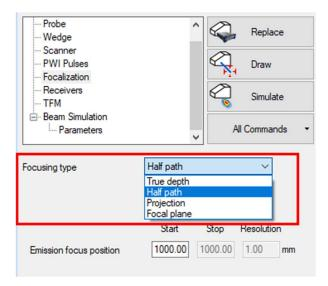
For the **Emission focus position**, the default setting is 1000 mm, which for most probe configurations corresponds to **natural focusing**, i.e. *"Plane Wave" excitation*. This is the recommended setting to perform PWI with pulse-echo configurations.
