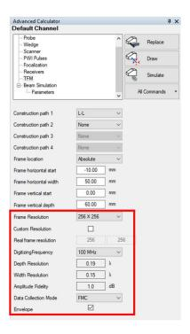
On the receiving side, a 256 by 256 TFM frame is selected. With the Envelope feature activated, this configuration provides an Amplitude Fidelity of 1.0 dB, well below the threshold of 2 dB required to be Code Compliant.
