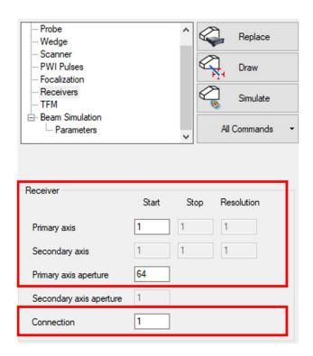
For a pitch & catch configuration, the default setting is the first element of the receiver probe, and depends on the wiring of the considered pitch & catch probe assembly.
