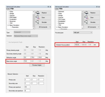
For the value of the **Beam skew angle**, a good starting point is to look at the standard PA UT configuration with the considered DMA probe, and observe the Advanced Calculator information for the skew angle in the **Transmitter** probe (105 degrees total skew – 90 degrees probe skew = 15 degrees beam skew).
