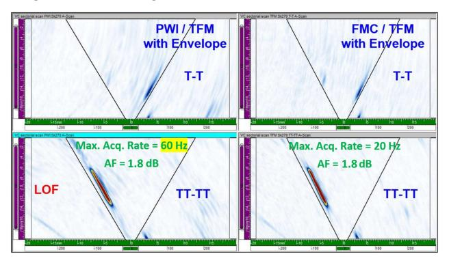
On the left side of the images, the T-T and TT-TT reconstruction modes from the PWI firing sequence are shown, and on the right the same wave modes for the regular FMC-TFM.
