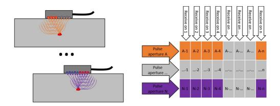
The receiving process is done with each element individually, and a TFM frame is processed from the raw data. Live PWI-TFM imaging is done during inspection, and the encoded data can be saved just like for regular phased array UT or live TFM.
