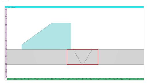
With the considered probe and wedge selection, the **Configuration PWI Pulse-Echo** is selected in the **Probe** tab of the Advanced Calculator, and the dedicated tabs for PWI appear.
