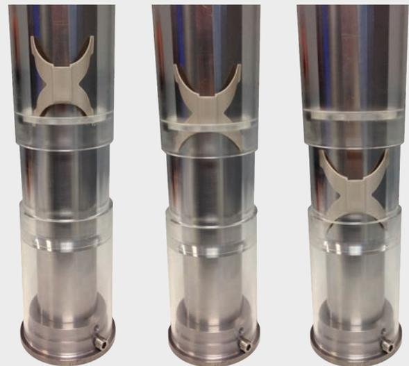
**Mock up of a thermal sleeve and transparent thermoplastic nozzle**
