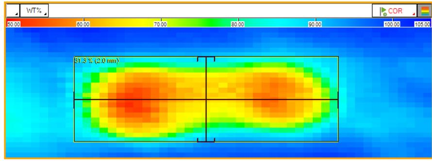
Examples of Compensated Wall Thickness
